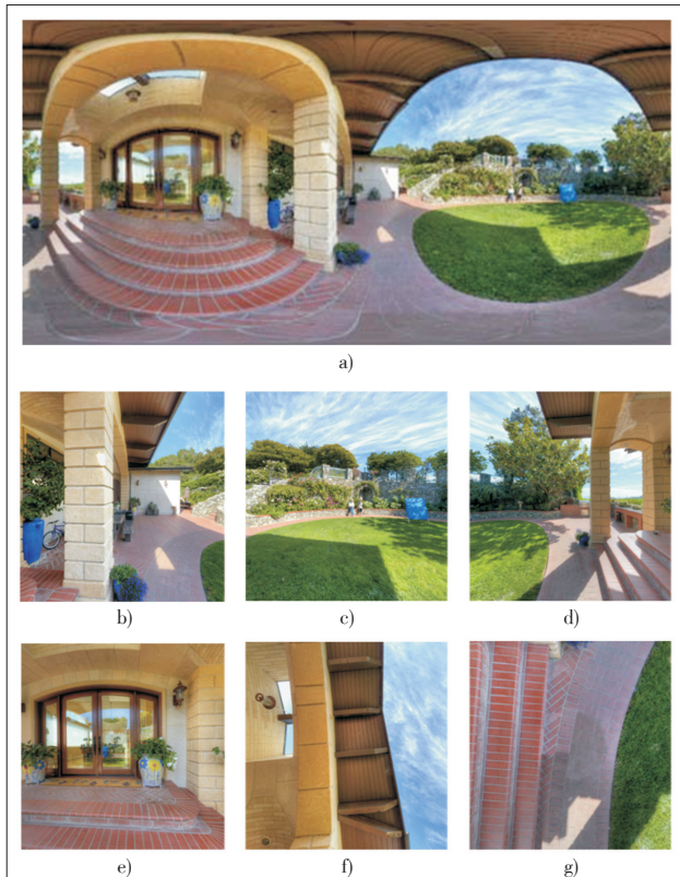
▲ Figure 7. Omnidirectional images of equirectangular format or cubic format: a) Equirectangular image; b)–g) cubic images, which are Front, Right, Back, Left, top and bottom in sequence.
