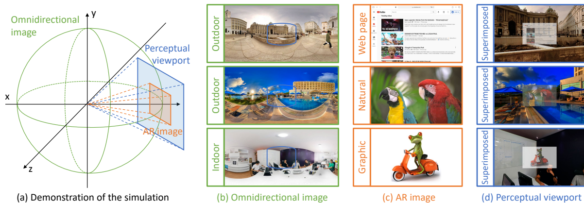
Fig. 2. The illustration of the AR simulation in VR environment. (a) The demonstration of the relationship between the omnidirectional image, the AR image, and the perceptual viewport image. (b) The omnidirectional images are used as the background scenes, which include outdoor and indoor scenarios. (c) The AR images are composed of three types of content including web page images, natural images, and graphic images. (d) The perceptual viewport images are generated by superimposing the AR images on the omnidirectional images (here \lambda = 0.58 ). Note that the perceptual viewports of the subjects are changed dynamically with the head movement, however, the relative positional relationship between the omnidirectional image and the AR image is fixed.
