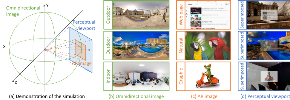
Fig. 12. The illustration of the AR simulation in VR environment. (a) The demonstration of the relationship between the omnidirectional image, the AR image, and the perceptual viewport image. (b) The omnidirectional images are used as the background scenes, which include outdoor and indoor scenarios. (c) The AR images are composed of three types of content including web page images, natural images, and graphic images. (d) The perceptual viewport images are generated by superimposing the AR images on the omnidirectional images (here \lambda = 0.58 ). Note that the perceptual viewports of the subjects are changed dynamically with the head movement, however, the relative positional relationship between the omnidirectional image and the AR image is fixed.
